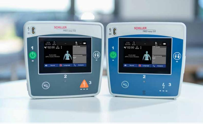
The choice is yours: FRED easy G2 is available as a semi-automatic version (device on the left) and a fully automatic version (device on the right).
