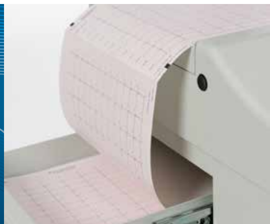
Built-in printer with 300-page paper capacity and integrated paper holder
